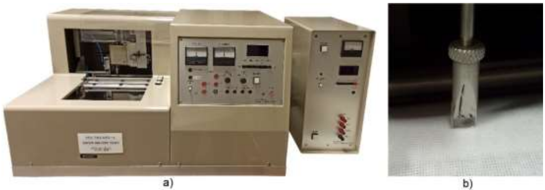
Figure 1. a) KES-FB4 AUTO instrument; b) Sensor for measuring geometric roughness
